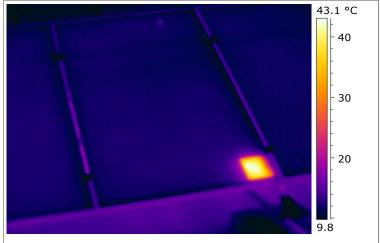
On this panel the defect is more pronounced. We can see, in this photo, darkening of the area in question. Replacement of the panel is necessary to reduce risk of fire and damage to other panels.
